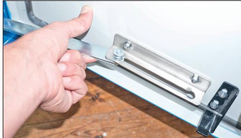
Fig. 18: releasing the locking rail
