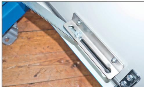
Fig. 19: released locking rail
