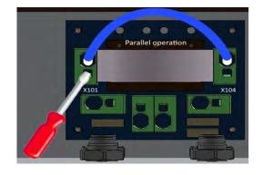
This section applies only, if several Strings with an equal amount of modules are to be connected in parallel and the maximum input current per input therefore exceeds 12A.
