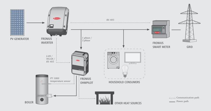
Installing the Fronius Ohmpilot could not be easier thanks to straightforward commissioning via the dedicated website as well as a simple communication connection via WLAN. The Fronius Ohmpilot also protects the grid by cleanly and reliably activating the consumers, leaving you as the installer fully equipped for the demands of today and tomorrow.
