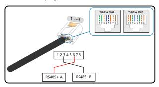
step 4 Insert the RJ45 connector to the RJ45 jack.
