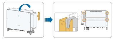
**step 4** Fix the inverter with screws.
