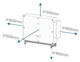
In case of multiple inverters, reserve specific clearance between the inverters.
