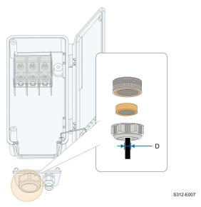
step 5 Install the cables and reinstall the bottom sealing plate.
