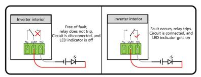
figure 5-8 Normal open contact
