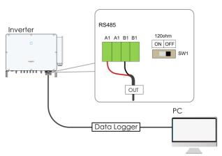
figure 5-5 Single-inverter Connection
