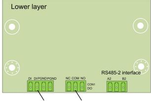
Emergency stop dry contact Fault output dry contact
