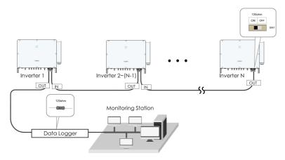
figure 5-7 Configuration of Dip Switch (N≥15)
