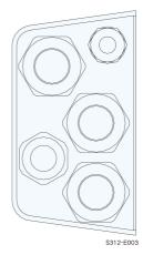
figure 5-2 Spare AC Sealing Plate
