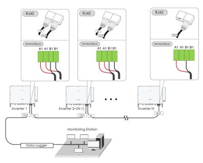
figure 5-6 Multi-inverter Connection
