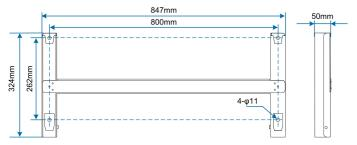
figure 4-1 Dimensions of mounting-bracket
