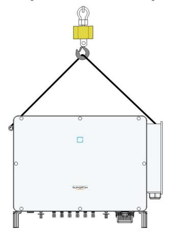
**step 4** Remove the lifting rings and reassemble the sealing screws released in Step 1.
