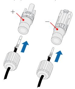
step 4 Check for polarity correctness.
