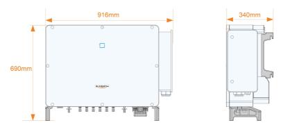
figure 2-3 Dimensions of the Inverter(in mm)
