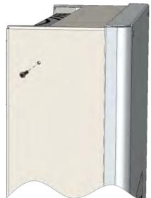
Loosen the inverter's left and right-sided locking screws at the top.
