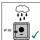
The inverter is suitable for outdoor installation.
