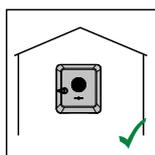
The inverter is suitable for indoor installation.
