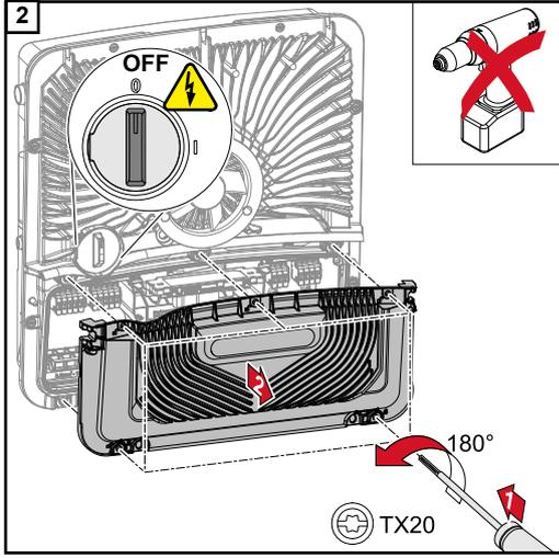
Loosen the five screws of the connection area cover by rotating them 180° to the left using a screwdriver (TX20). Remove the connection area cover from the device.
