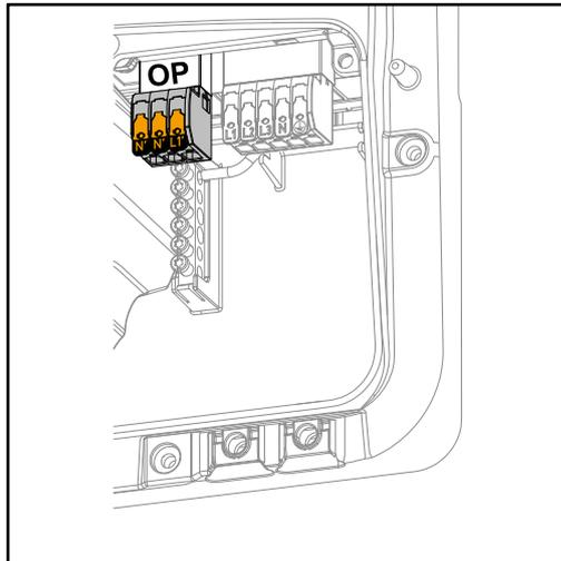
With the PV Point, in the event of a failure of the public grid, single-phase electrical devices can be connected to the Opportunity Power (OP) terminal and supplied with a maximum power of 3 kW, if enough power is available from the solar modules or an optional battery. In grid-connected operation, the OP terminal is not supplied with voltage, therefore the connected loads will not be supplied with power in this operating mode.
