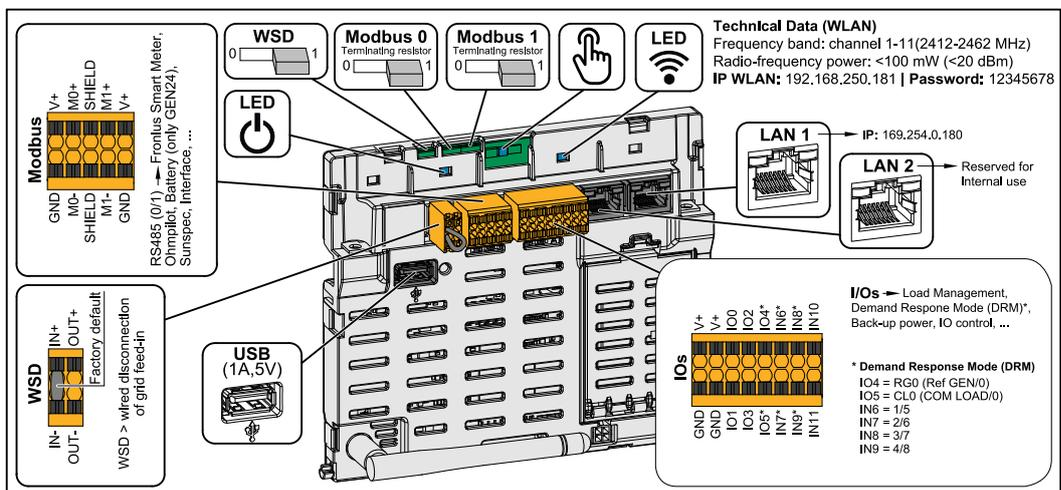
Push-in terminal for the installation of Modbus 0, Modbus 1, 12 V and GND (ground).
