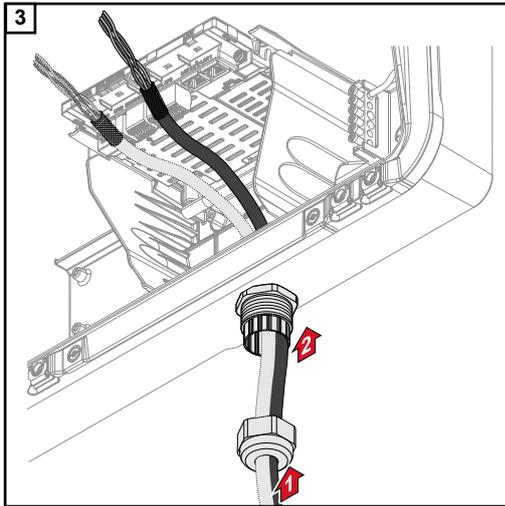
Guide the data cables first through the strain-relief device union nut and then through the housing opening.
