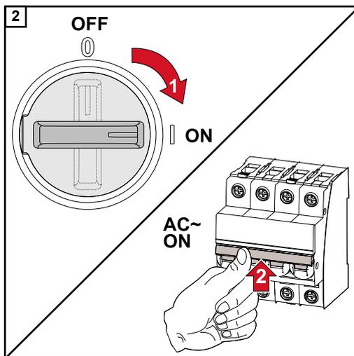
Set the DC disconnect to the "On" switch position. Switch on the automatic circuit breaker.
