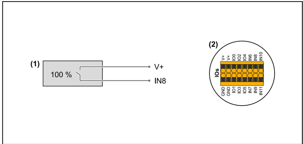
(1) Ripple control signal receiver with 1 relay, for effective power limiting.
