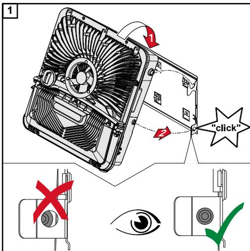
Clip the inverter into the mounting bracket from above. The connections must point downwards.
