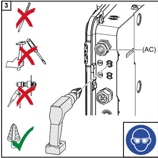
Drill out the optional cable guide with a step drill.
