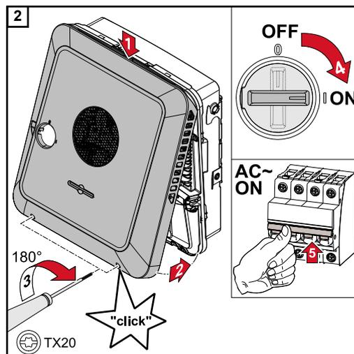
Clip the housing cover onto the inverter from above. Press on the lower part of the housing cover and tighten the two screws 180° to the right using a Torx screwdriver (TX20). Turn the DC disconnecter to the "On" switch position. Switch on the automatic circuit breaker. For systems with a battery, observe the switch-on sequence according to chapter [Suitable battery](#) on page 22.
