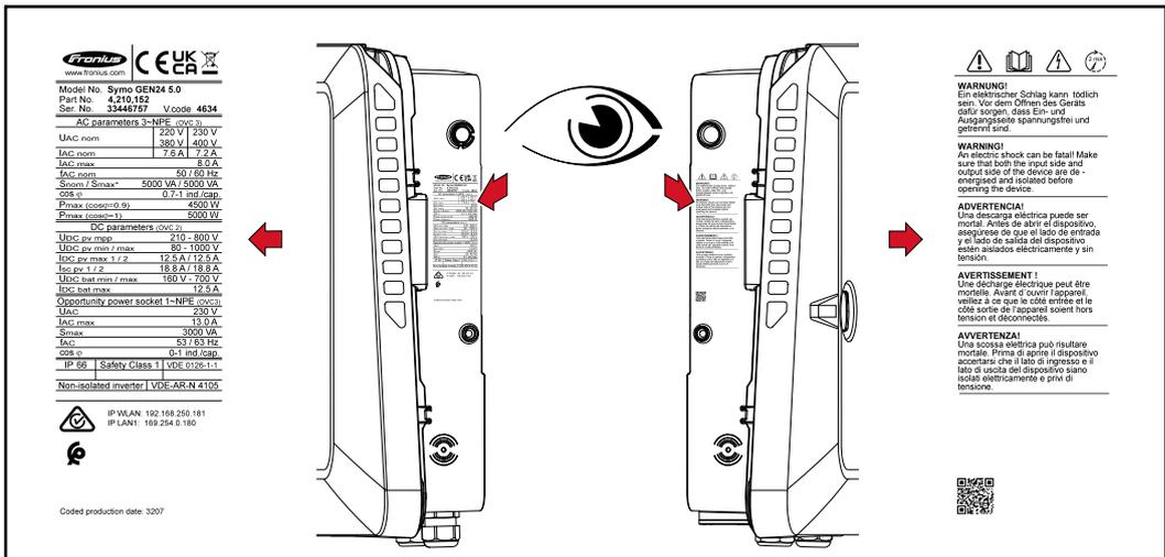
A 4-digit number (coded production date) is printed on the rating plate at the very bottom, from which the production date can be calculated.
