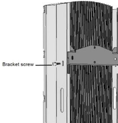
Figure 8: Inserting the bracket screws
