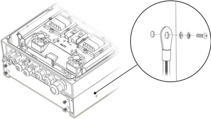
Figure 18: Grounding the battery
