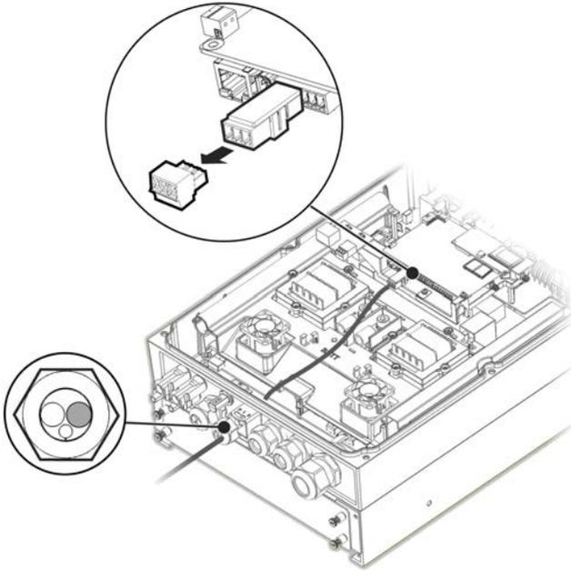
Figure 13: Meter Connection
