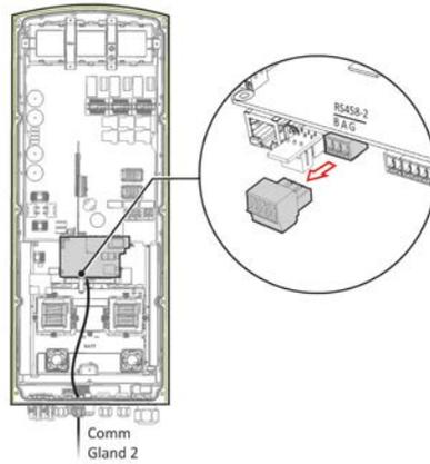
Figure 22: RS485 connector on the communication board
