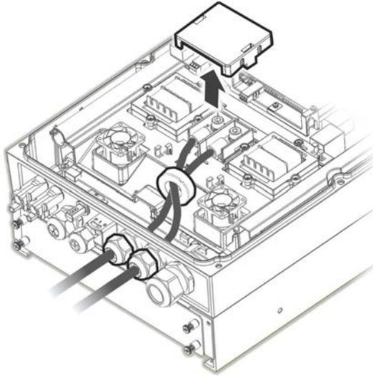
Figure 15: Connection of Battery DC Cables to the Inverter
