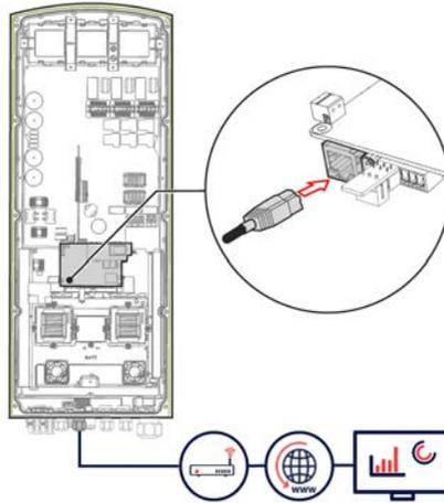
Figure 21: RJ45 Ethernet connection
