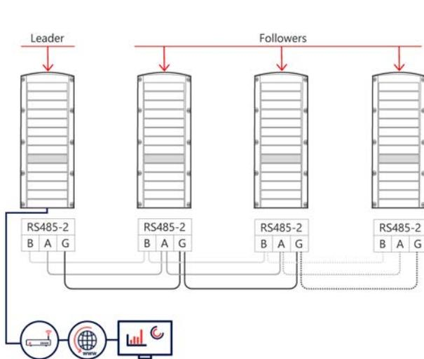
Figure 23: Connecting the inverters in a chain
