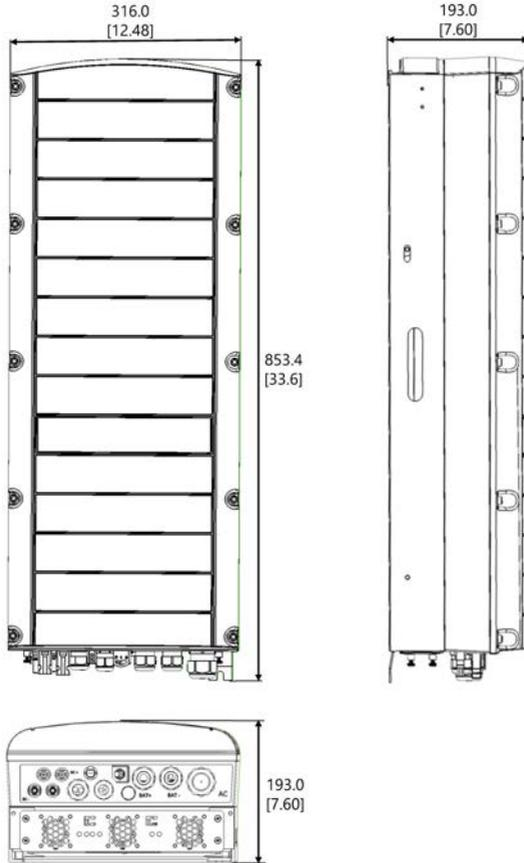
Figure 25: StorEdge Three Phase Inverter dimensions
