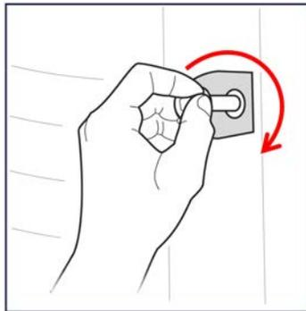
3. Fasten all bolts to a torque of 4 N\*m in the order, shown below.
