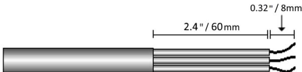
Figure 10: Insulation Stripping – AC Cable
