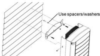
5. Hang the inverter on the bracket (see *Figure 7*): Lift the inverter from the sides, or hold it at the top and bottom of the inverter to lift the unit into place.
