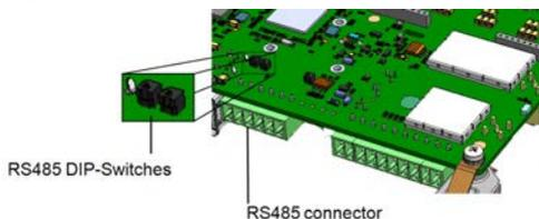
Figure 24: RS485 termination switch
