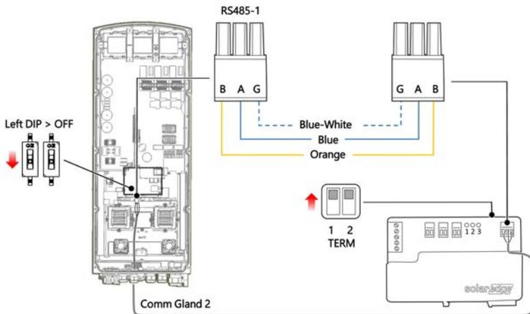
Figure 14: Meter Connection 2
