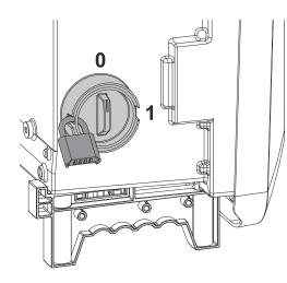
The DC disconnector has 2 switch settings: On / Off.
