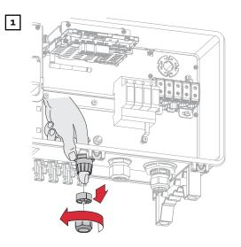
Undo the cable gland union nut and push out the sealing ring and the blanking plug from the inside of the device.
