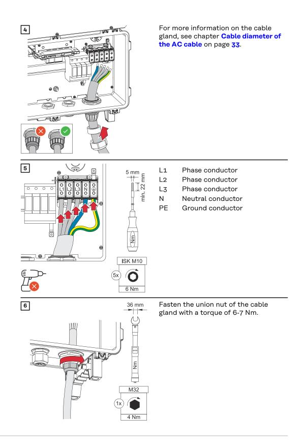
Connecting the inverter to the public grid with the PEN conductor (AC side) It is not possible to operate the inverter in unearthed grids, such as IT grids (insulated grids without ground conductor).
