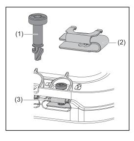
A quick-lock system (3) is used to mount the connection area cover and front cover. The system is opened and closed with a half-rotation (180°) of the captive screw (1) into the quicklock spring (2).
