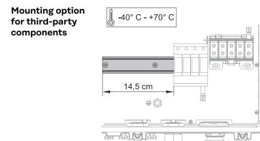
In the connection area there is space for mounting third-party components. Components up to a maximum width of 14.5 cm (8 DU) can be mounted on the DIN rail. The components must have a temperature resistance of -40 °C to +70 °C.
