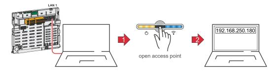
**1** Establish a connection to the inverter (LAN1) with a network cable (CAT5 STP or higher).
