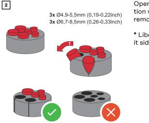
Open up the sealing ring at the location where the blanking plug is to be removed.
