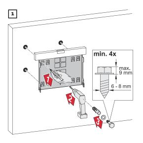
Attaching the inverter to the mounting bracket
