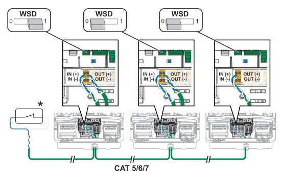
\* Floating contact of the trigger device (e.g. central grid and system protection). If several floating contacts are used in a WSD chain, they must be connected in series.
