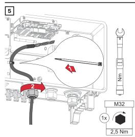
Secure the data cable to the protective cover of the DC SPD surge protective device with a cable tie. Tighten the union nut for the cable gland to a torque of min. 2.5 to max. 4 Nm. Installing the WSD (wired shutdown)
