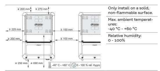
When installing the inverter in a switch cabinet or similar closed environment, it is necessary to make sure that the hot air that develops will be dissipated by forced-air ventilation.
