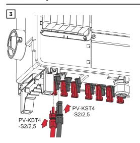
Connect the PV cables from the solar modules to the MC4 connectors as labelled.
