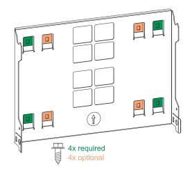
The mounting bracket (illustration) can also be used as a guide.
