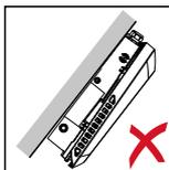
Do not install the inverter overhanging with the connection sockets at the top.
