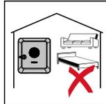
During certain operating phases the inverter may produce a slight noise. For this reason it should not be installed in an occupied living area.
