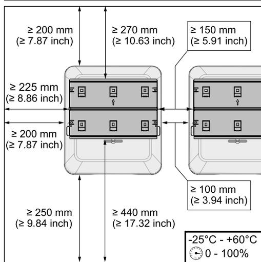
Only install on a solid, non-flammable surface.
