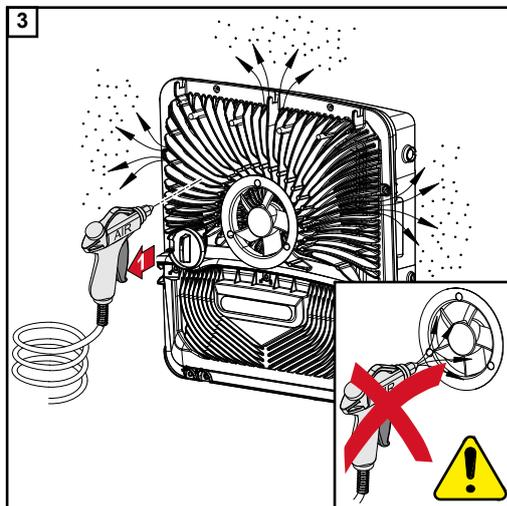
Remove any build-up of dirt on the heat sink and fan using compressed air, a cloth, or a brush.
