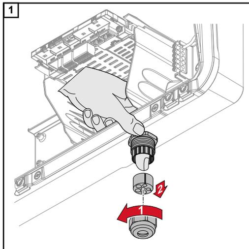
Undo the strain-relief device union nut and push out the sealing ring and the blanking plug from the inside of the device.
