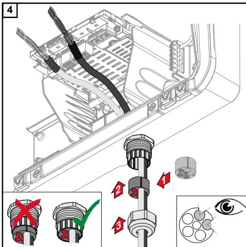
Insert the sealing ring between the union nut and the housing opening. Press the data cables into the seal's cable guide. Then press in the seal until it reaches the underside of the strain-relief device.
