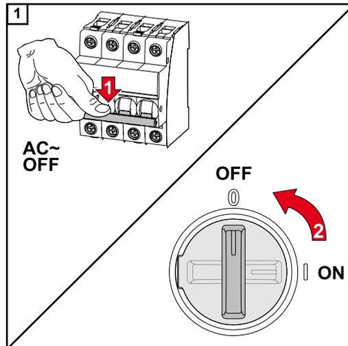
Turn off the automatic circuit breaker. Set the DC disconnector to the "Off" switch position.
