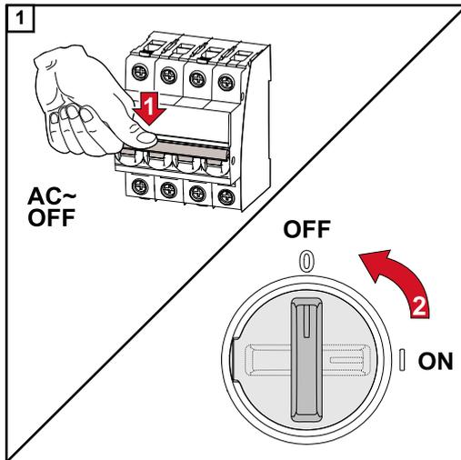
Switch off power to the inverter and wait for the specified time (2 minutes) until the capacitors have discharged and the fan has shut down.
