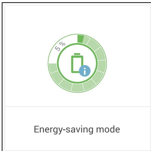
Energy saving mode is shown on the website of the inverter and in Solar.web by an "i" beside the battery symbol in the system overview.
