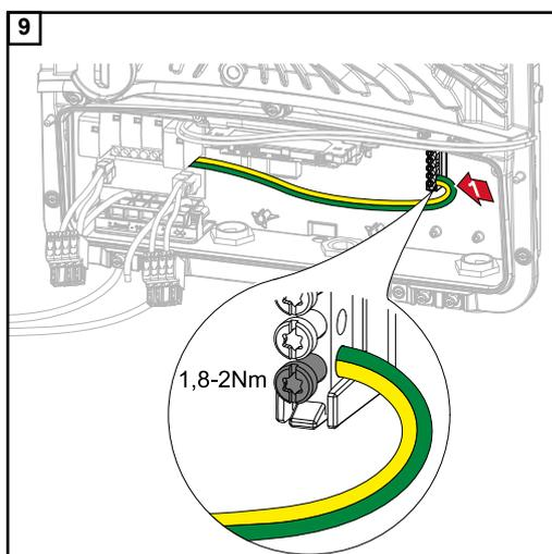
Fasten the ground conductor to the first input from the bottom of the ground electrode terminal using a screwdriver (TX20) and a torque of 1.8 - 2 Nm.
