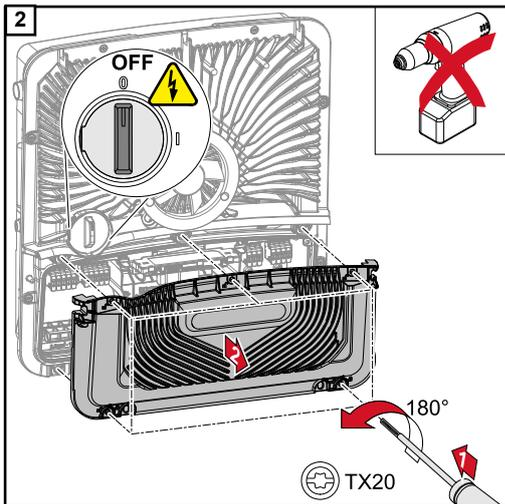
Make sure that the DC disconnect is in the "Off" switch setting.
