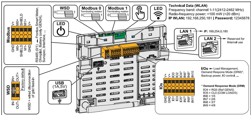
Push-in terminal for the installation of Modbus 0, Modbus 1, 12 V and GND (ground).
