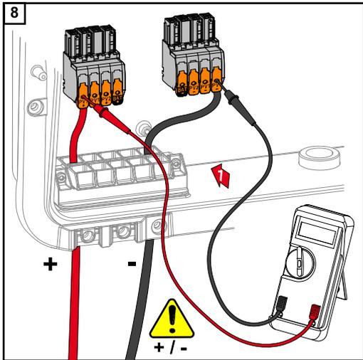
Use a suitable measuring instrument to check the voltage and polarity of the DC cabling. Remove both DC terminals from the slots.
