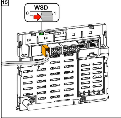
Check whether the WSD switch is in position 1, adjust if necessary (factory setting: position 1).
