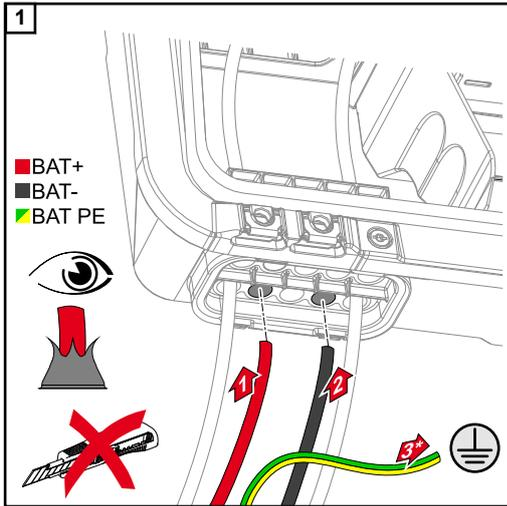
Manually push the BAT cables through the DC bushings.
