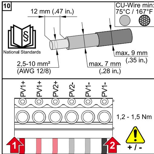
Strip the insulation on the single conductors by 12 mm and secure to the corresponding slot of the terminal on the PC board with a torque of 1.2 - 1.5 Nm.
