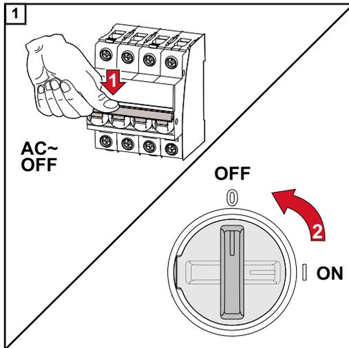
Switch off the automatic circuit breaker and DC disconnect.
