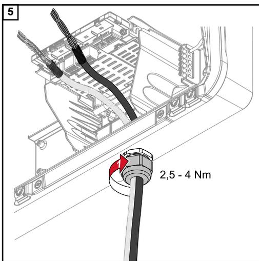
Fasten the union nut of the strain-relief device with a torque of min. 2.5 - max. 4 Nm.
