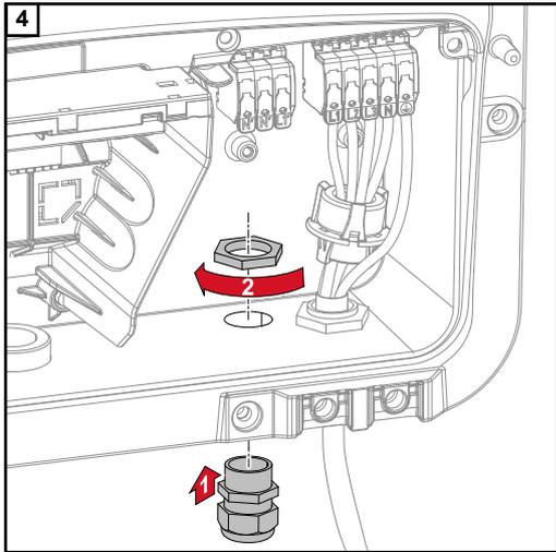
Insert the strain-relief device into the hole and secure to the torque specified by the manufacturer.
