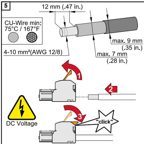
Select the cable cross section in accordance with the instructions in **Permitted cables** from page 45.
