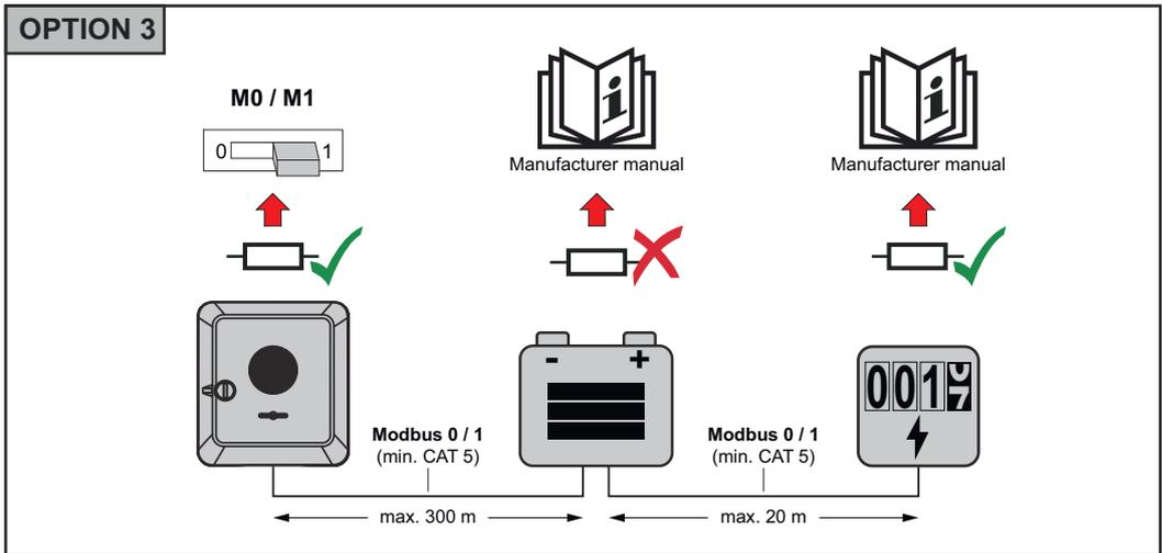
**Installing the WSD (wired shut-down)**
