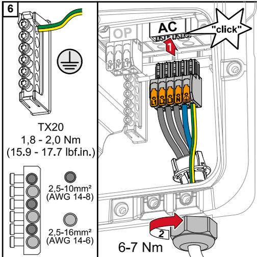
Insert the AC terminal into the AC slot until it engages. Fasten the union nut of the strain-relief device with a torque of 6-7 Nm.
