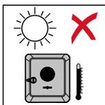
In order to minimise the heating up of the inverter, do not expose it to direct insolation. The inverter should be installed in a protected location, for example, near the solar modules or under an overhanging roof.
