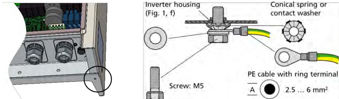
Fig. 5-6 Material not included in scope of supply.
