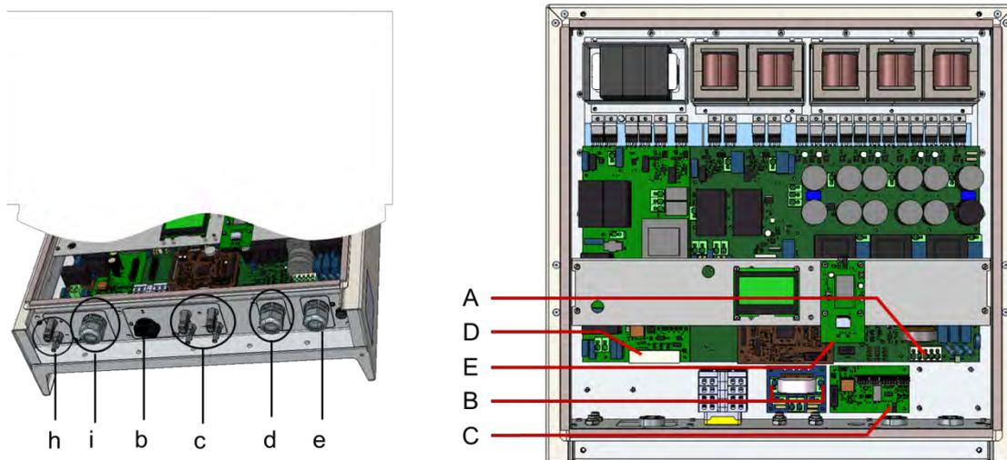
Fig. 5-1 Overview of wiring area and interior connecting components
