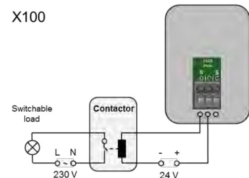
Fig. 6-4 Connection - Contactor and switchable load
