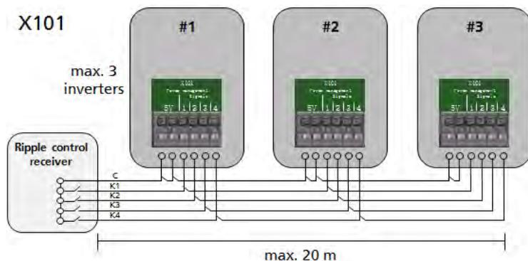
Fig. 6-5 Connection - Ripple control receiver
