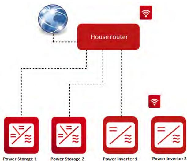
Fig 2: Device networking via router [4 clients]
