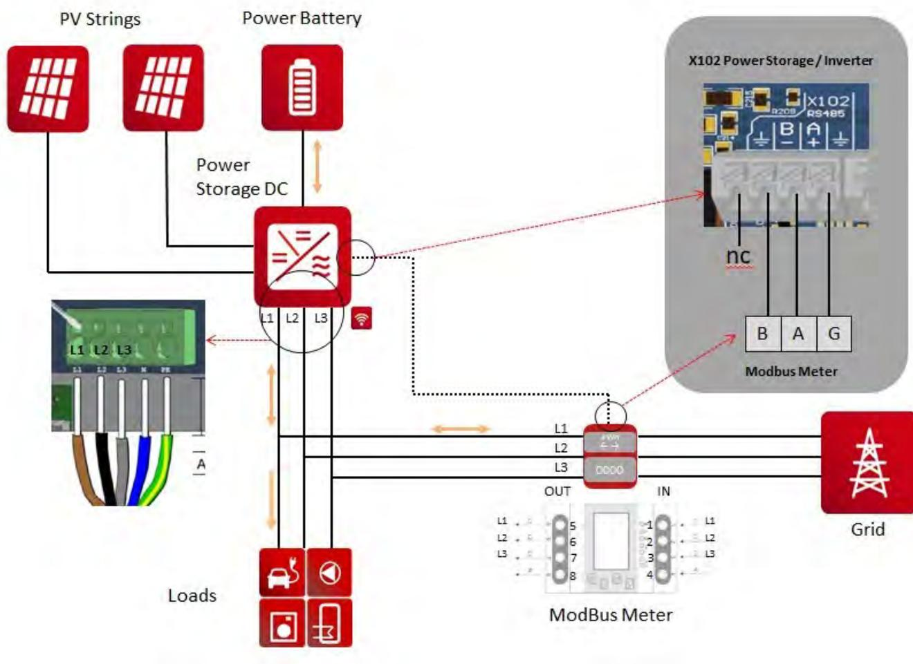
**Modbus connected meter with radio transmitter module:**
