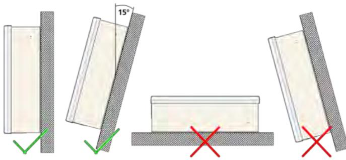
Mount the inverter in an upright or slightly backward inclined position.
