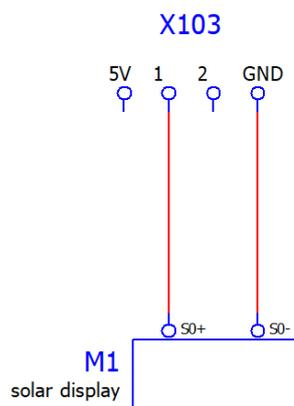
Please configure the appropriate pulse ratio of the solar display in the RCT Power APP.
