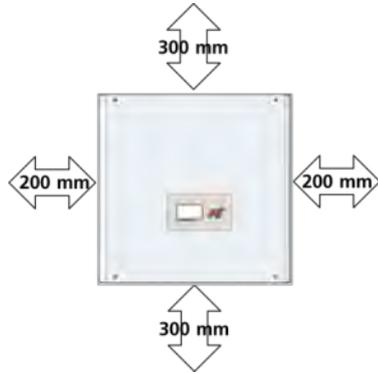
Required minimum distances to allow sufficient free convection of air for cooling the unit.
