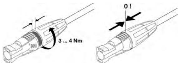
Turn connector plug in screw fitting.
