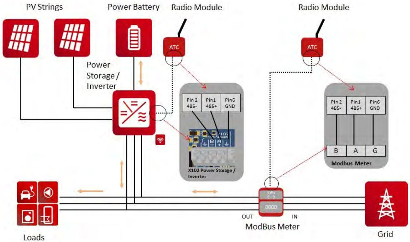
Please note: Radio transmission connection requires an auxiliary power supply (plug-in power supply unit included in the scope of supply).
