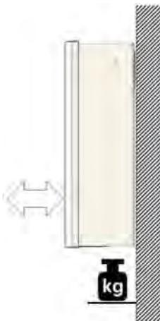
The mounting surface must be solid and able to permanently support the weight of the inverter unit.
