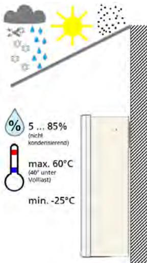
The inverter must be protected from dust, snow, rain and direct thermal radiation (e.g. solar radiation, central heating radiators, etc.).
