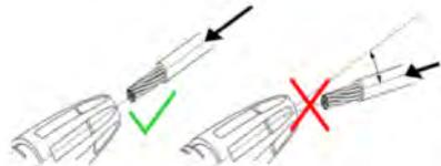
Insert the cable in a straight line into the plug.
