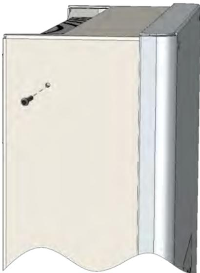
Loosen the inverter's left and right-sided locking screws at the top.
