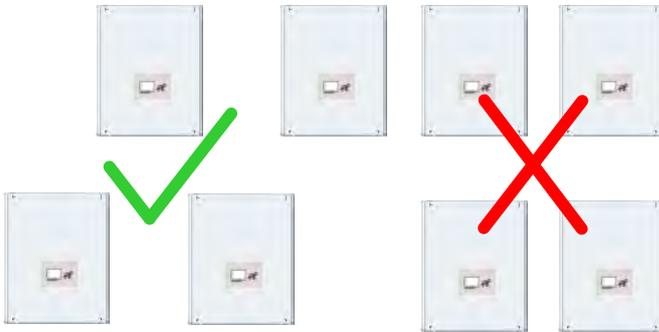
To prevent mutual heating, inverters must not be mounted on top of each other.
