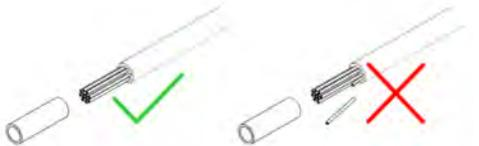
Remove the cable insulation carefully.
