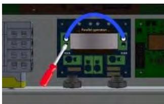
Remove the inverter cover. Identify the terminals for parallel operation.
