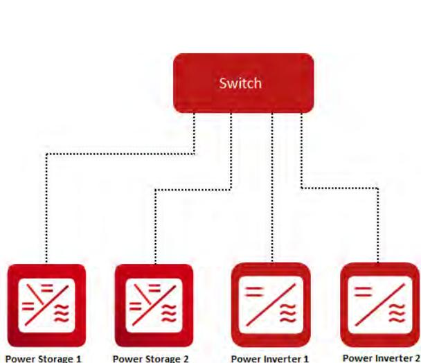
Fig. 1: Device networking via switch [4 clients]
