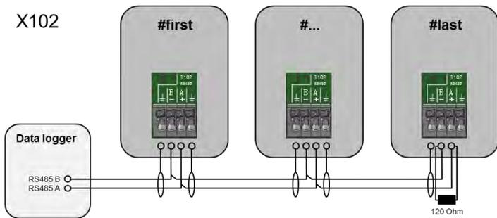
Fig. 6-3 Connection of data logger
