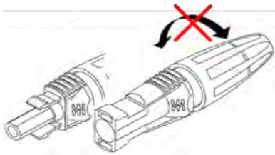
Do not turn connector plug in the screw fitting before strands are wired.
