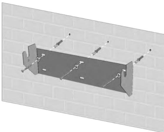
Mount the wall bracket as shown left. Use at least 3 screws ( $\varnothing$  6-8mm), 3 washers (outside  $\varnothing$  min. 18mm) and the appropriate dowels.
