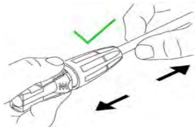
Check that the connection has snapped in correctly with a slight pull on the cable.
