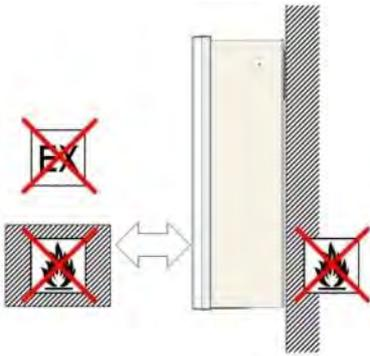
The mounting surface must be made of flame-retardant material.
