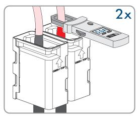
9. Ensure that no voltage is present between the positive terminal and negative terminal on the DC surge protection devices using a suitable measuring device. To do so, insert the test probe (maximum diameter: 2.5 mm) into the measuring points of the DC surge protection devices.
