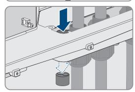
For each network cable, remove one of the plugs from the cable support sleeve and cut the enclosure opening laterally with a utility knife. This will push the cable into the opening.
