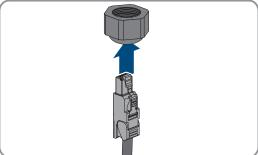
4. Remove the two-hole cable support sleeve from the cable gland.
