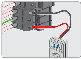
10. Ensure that no voltage is present between the positive terminal and ground as well as between the negative terminal and ground on the DC surge protection devices using a suitable measuring device. To do so, insert a test probe (maximum diameter: 2.5 mm) into the measuring points of the DC surge protection devices and hold the other one, for example, on the enclosure.
