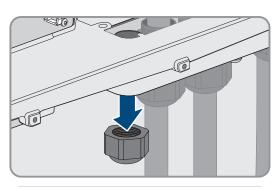
3. Thread a swivel nut over each network cable.
