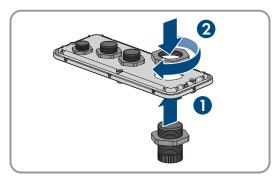
Lead the cables through the cable glands in the connecting plate and align the connecting plate by means of the mounting template.
