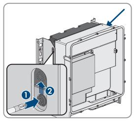
3. Move the fan bracket upwards and fold it backwards. When doing this, note that the fan bracket cannot be removed completely, because the fan cable connects it to the product.
