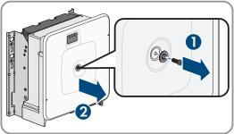
6. Set the cover, screw with seal, washer with seal and enclosure lid aside and store safely.
