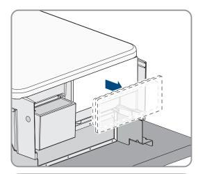
5. Secure the pre-configured DC connection cables in the defective product for transport. To do so, screw the supplied cable tie into the hole below the DC surge protection devices and place and tighten the cable tie around the DC connection cables.
