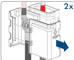
4. Remove the DC cable connection. Loosen the hex nuts and remove the combined hexagon head screw (AF16).
