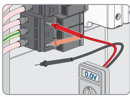
11. Ensure that no voltage is present on the AC terminal block between L1 and grounding conductor, L2 and grounding conductor, and L3 and grounding conductor using a suitable measuring device. To do so, insert the test probe (maximum diameter: 2.5 mm) into the measuring points of the respective terminal blocks.
