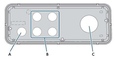
Figure 7: Overview of the connecting plates that can be ordered as an accessory
