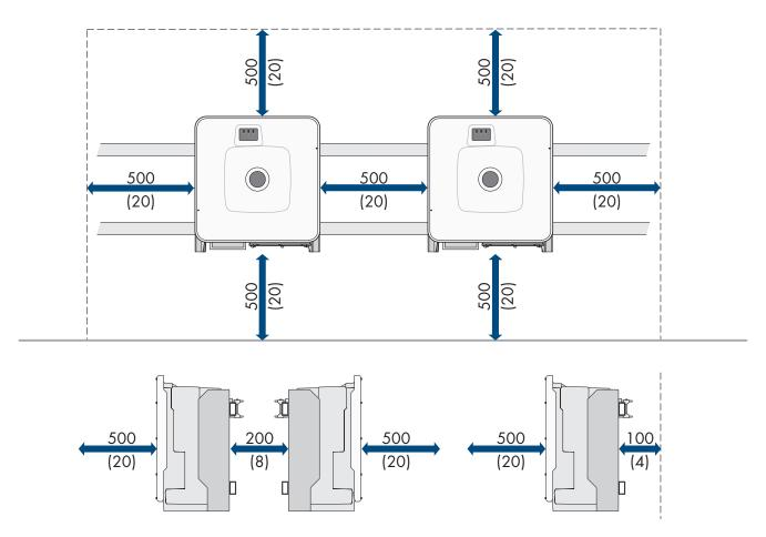
Figure 5: Recommended clearances (dimensions in mm (in))
