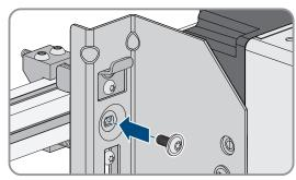
10. Remove all 4 transport handles from the tapped holes. If necessary, insert a screwdriver into the holes on the transport handle and use the screwdriver to remove the transport handle.
