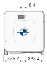
Figure 8: Dimensions of the center of gravity of the product (dimensions in mm (in))
