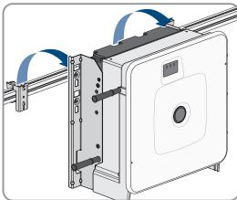
Remove all 4 transport handles from the tapped holes. If necessary, insert a screwdriver into the holes on the transport handle and use the screwdriver to remove the transport handle.
