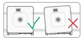
10. Hold the enclosure lid pressed against the enclosure and screw and tighten the screw (hex socket AF8, torque: 18 Nm).
