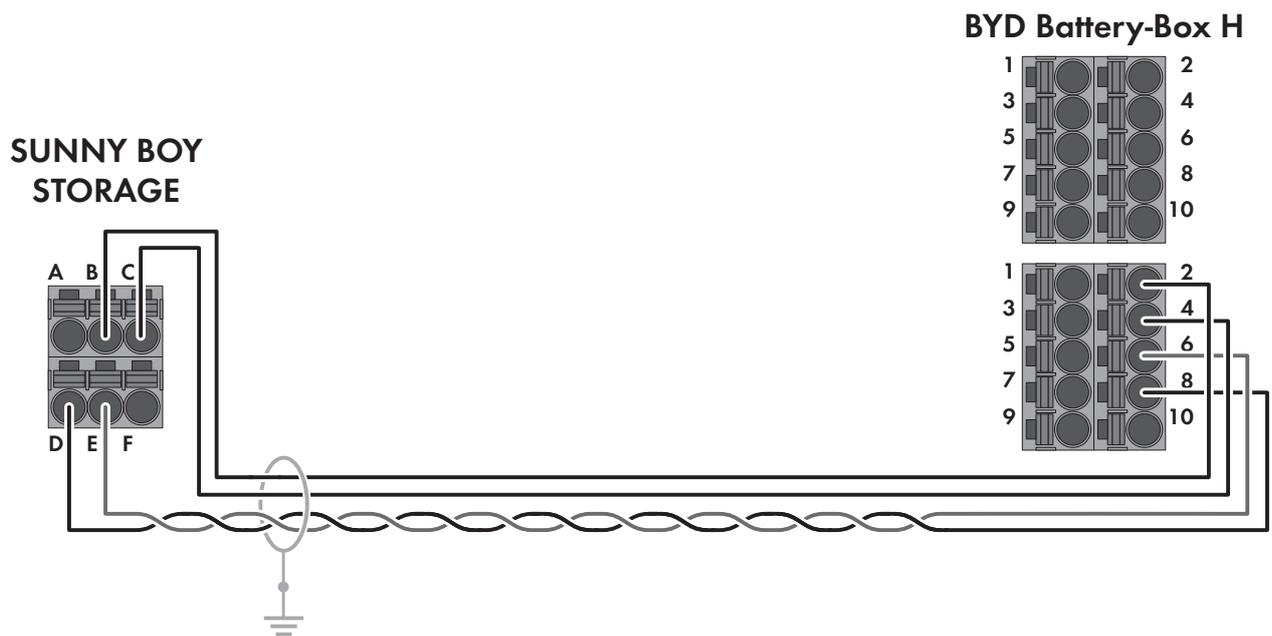
Figure 8: Cabling plan SBS3.7-10 / SBS5.0-10 / SBS6.0-10 with Battery-Box H
