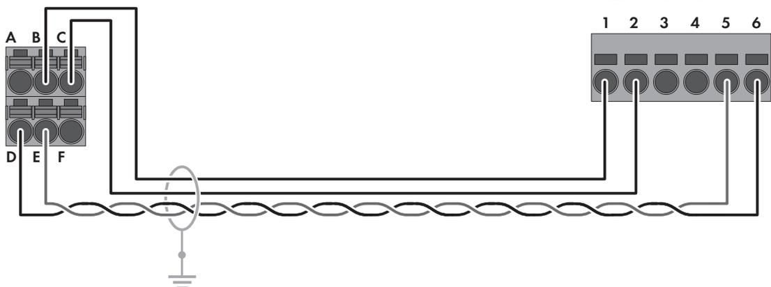
Figure 13: Cabling plan SBS3.8-US-10 / SBS5.0-US-10 / SBS6.0-US-10 with RESU 16H Prime
