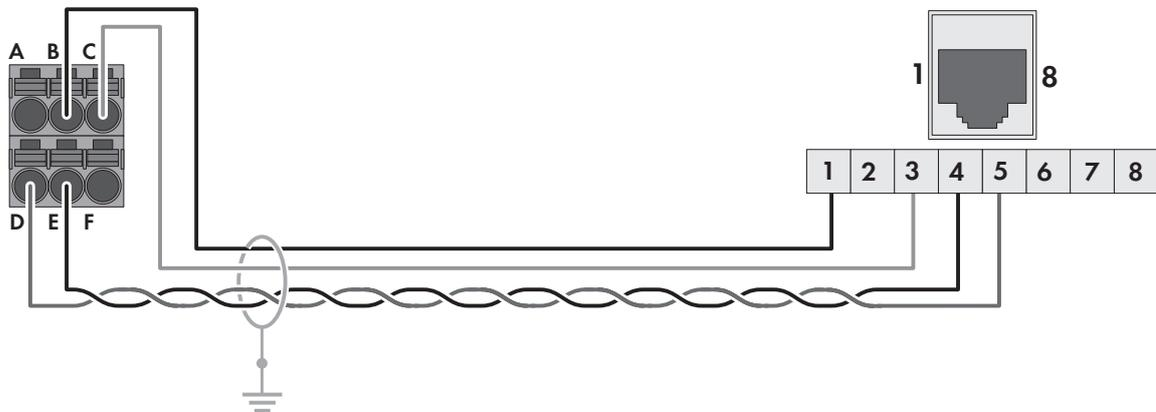
Figure 5: Cabling plan SBS3.7-10 with RESU 10M
