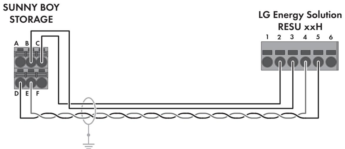
Figure 11: Cabling plan SBS3.8-US-10 / SBS5.0-US-10 / SBS6.0-US-10 with RESU 7H / RESU 10H
