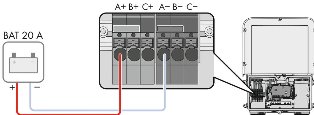
Figure 14: Overview for connection of a battery with a charging/discharging current limit of 20 A
