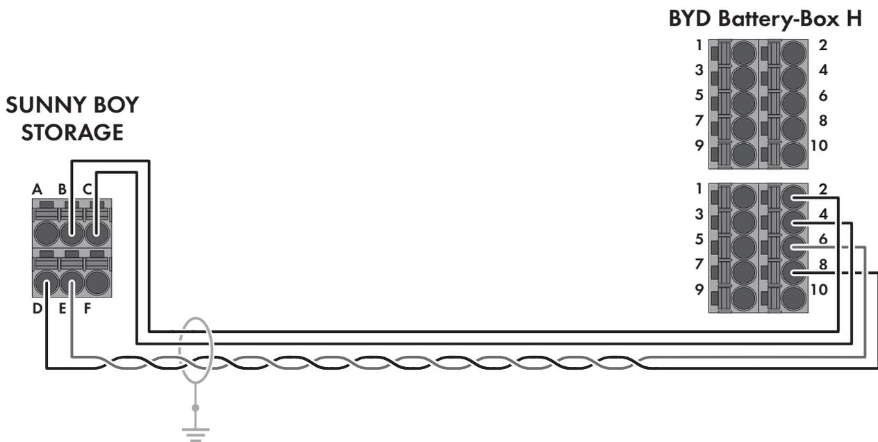
Figure 12: Cabling plan SBS3.8-US-10 / SBS5.0-US-10 / SBS6.0-US-10 with BYD Battery-Box H
