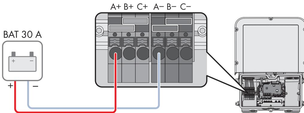
Figure 15: Overview for connection of one battery with a charging/discharging current higher than 20 A.
