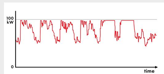
\* Data relating to the sample property: Medium-sized supermarket (aktiv&irma) in Oldenburg, Germany; planned energy system: PV system (199 kWp) with self-consumption; battery-storage system for load peak capping (Sunny Tripower Storage 60, SMA Storage Business (14 modules), 67 kWh). Details regarding the simulation of the SMA Energy System "Business XL" can be found online at [go.sma.de/SESde](http://go.sma.de/SESde).
