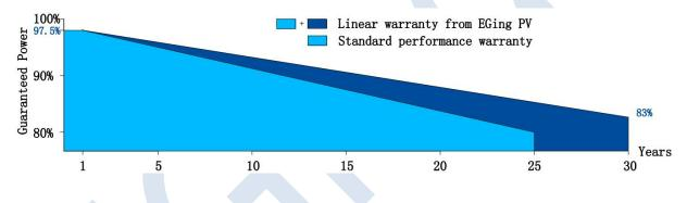
(4)For Monocrystalline double glass modules: not exceed 2.5% degradation in the first year, and 0.5% per year thereafter, ending at 83% in the 30th year after warranty start.
