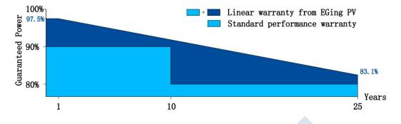
(3)For Polycrystalline double glass modules: not exceed 2.5% degradation in the first year, and 0.5 % per year thereafter, ending at 83% in the 30th year after warranty start.
