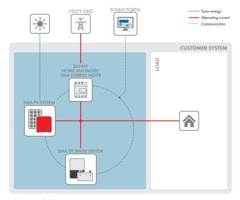
Figure 3: Design of the system
