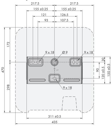
Figure 7: Position of the anchoring points(Dimensions in mm)
