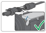
4. If the stranded wire is not visible in the chamber, the cable is not correctly inserted and the connector must be reassembled. To do this, the cable must be removed from the connector.  Release the clamping bracket. To do so, insert a screwdriver (blade width: 3.5 mm) into the clamping bracket and pry the clamping bracket open.
