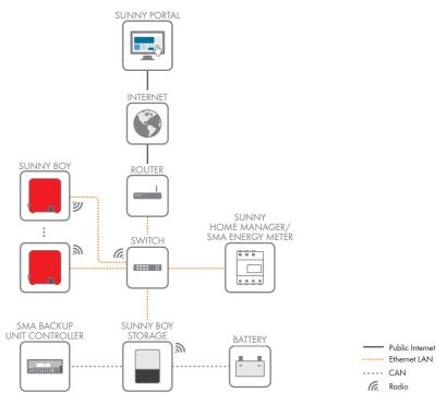
Figure 5: Design of system communication
