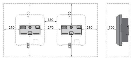
Figure 8: Recommended clearances (Dimensions in mm)
