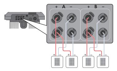
Figure 10: Connection overview for normal operation
