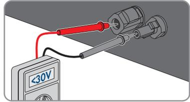
8. Ensure that no voltage is present between the positive terminal and ground as well as between the negative terminal and ground on the DC inputs using a suitable measuring device.
