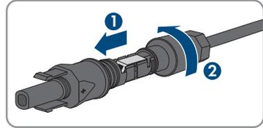
5. Push the swivel nut up to the thread and tighten (torque: 2 Nm).
