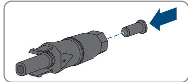
12. Insert the DC connectors with sealing plugs into the corresponding DC inputs on the inverter.
