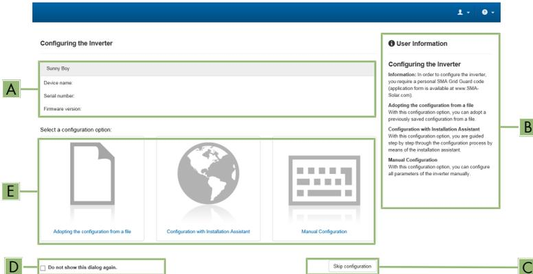
Figure 13: Layout of the **Configuring the Inverter** page
