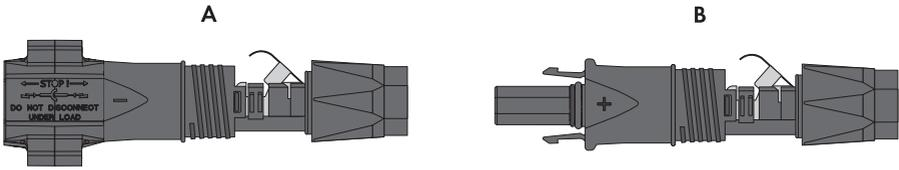
Figure 12: Negative (A) and positive (B) DC connectors
