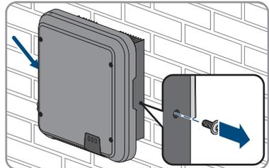
15. Remove the inverter by lifting it vertically up and off the wall mounting bracket.
