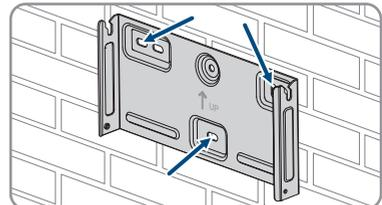
2. Set the wall mounting bracket aside and drill the marked holes.
