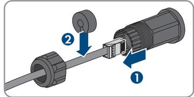
5. Press the cable support sleeve into the threaded sleeve.
