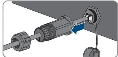
8. Take the cable support sleeve out of the threaded sleeve and remove the network cable from the cable support sleeve.
