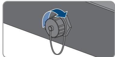
11. Unscrew and remove the antenna.
