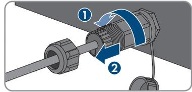
7. Release the network cable plug and pull it out of the jack on the inverter.
