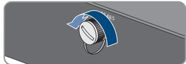
5. Plug the M12 connector into the jack for the RS485 communication connection and screw tight. When doing so, align the connector so that the key on the inverter AC jack is inserted into the keyway on the plug.
