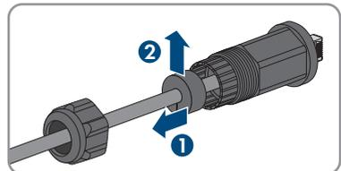
9. Lead the network cable out of the threaded sleeve and the swivel nut.
