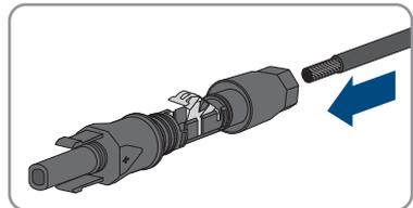
3. Press the clamping bracket down until it audibly snaps into place.
