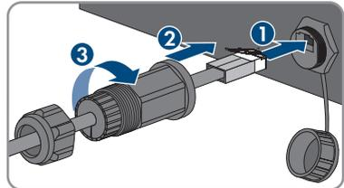
7. Screw the swivel nut onto the threaded sleeve.
