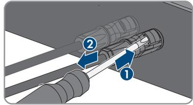
3. Unlock the DC connector. To do this, insert a flat-blade screwdriver (blade width: 3.5 mm) into the side catch mechanism and pry the catch mechanism open.
