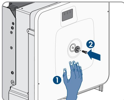
13. Place the cover on the screw in the enclosure lid.
