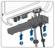
16. Screw the swivel nuts onto the cable glands on the connection cap.
