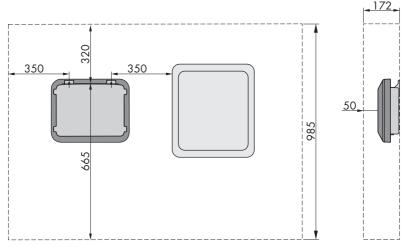
Figure 9: Recommended clearances(Dimensions in mm)
