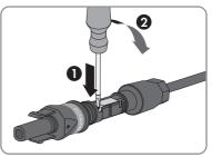
• Remove the cable and go back to step 2.
