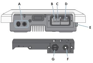
Figure 10: Connection areas at the bottom of the inverter and cable glands at the connection cap
