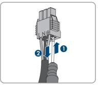
6. Tighten the connection cap with the three screws (TX20, torque: 3.5 Nm).
