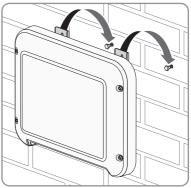
Tighten the screws hand-tight using a ratchet or box wrench. When doing this you can compensate for any misalignment of the drill holes by aligning the metal brackets accordingly.
