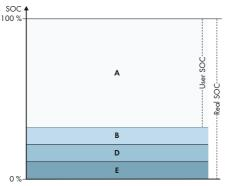
Figure 6: State of charge ranges of the battery in systems for increased self-consumption without battery backup
