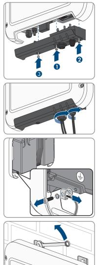
10. Remove the inverter from the screws using the metal brackets.
